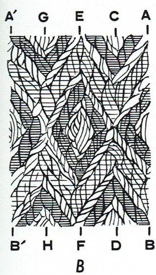
A Figure 63. Plaiting with thirty-eight strands of four colors and varying thickness producing square cross section. A: 1-9, successive positions of the strands; B: pattern formed by the movements
